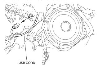
14. Disconnect the connector as shown.
