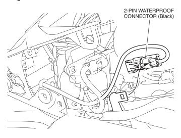
18. Remove the clip and disconnect the connector as shown.
